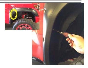
**STEP 7:** Using a 10mm socket / wrench, remove the 2 front screws from the inner splashguard front fascia area, retain these for later re-install.
