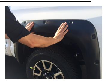
**STEP 15:** Hold Fender Flare on the vehicle in the position of best fit. Note where all the slots in the Fender Flare align with existing mounting holes in the vehicle.
