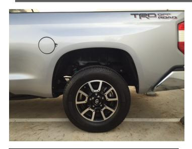
**STEP 14:** Clean the body area where the Fender Flares will make contact. Ensure fenders are dry prior to install.
