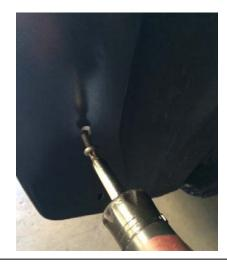
**STEP 9:** Working from top to bottom at the previously removed mud guard area, carefully hold and slide the supplied spacers in behind the Fender Flare to fill the gap between flare and fender. While holding the spacer, use your other hand to place the provided long screws through the slot and into the corresponding factory attachment points. Do not fully tighten screws at this stage.
