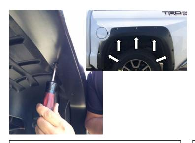
**STEP 16:** Loosely install a provided short screw into the top center hole in the Fender Flare. Continue installing the remaining (4) short screws into the 2 closest mounting locations either side of the top center hole. Do not fully tighten screws at this stage.
