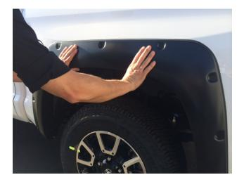
**STEP 18:** Working from top to bottom at these same (3) slot positions, hold and align the spacers with the slots and use the Long Screws to go through the spacers and into the corresponding factory holes.
