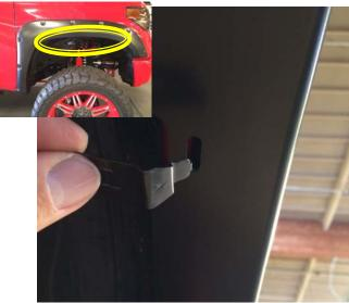
**STEP 10:** Locate the (3) remaining mounting slots on the Fender Flare as shown.
