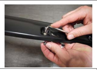
**STEP 1:** Attach the bolts, nuts and washers to each Fender Flare using a 5/32" Allen key and a 3/8" wrench/socket (wrench /socket and Allen key not supplied). Ensure inside of Fender Flares where the rubber seal is attached is clean, using the alcohol wipes provided. Wipe away any residue with a dry clean cloth.
